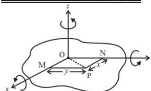
Let us consider a rigid laminar object able to rotate about three mutually perpendicular axes x, y and z. Let x and y axis be in the plane and z axis perpendicular to the plane. All 3 axes meet at O. Let dm be the mass at point P. x and y
