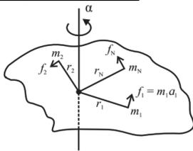
Let the object consists of N particles of mass  $m_1, m_2, \dots, m_N$  at respective perpendicular distance of  $r_1, r_2, \dots, r_N$  from the axis of rotation. As the rigid body is rotating, all these particles are performing CM with constant angular acceleration  $\alpha$  about an axis perpendicular to the plane of paper.
