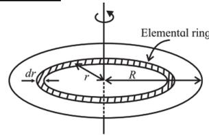
Consider a disc of mass M and negligible thickness and radius R. Let the axis of rotation pass through the center of the disc and perpendicular to it place. Let  $\sigma = \frac{M}{A} = \frac{M}{\pi R^2}$  be uniform. A disc can be considered a sequence of
