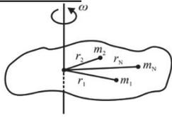
Let the object consists of N particles of mass  $m_1, m_2, \dots, m_N$  at respective perpendicular distance of  $r_1, r_2, \dots, r_N$  from the axis of rotation. As the rigid body is rotating, all these particles are performing UCM with constant angular speed  $\omega$  about
